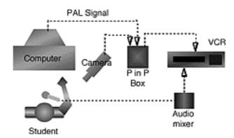
Figure 7: Connection diagram for video observation system
